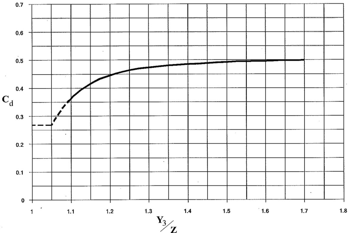
Figure 10: Bridge under Sluice Gate Type of Pressure Flow (after USACE, 2002)
