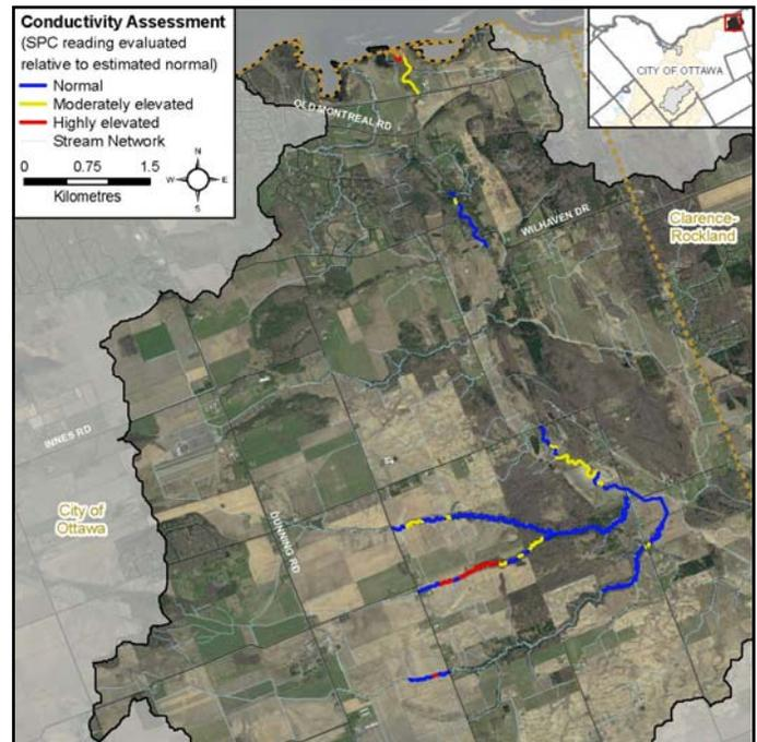
Figure 26 Relative specific conductivity levels along Becketts Creek
