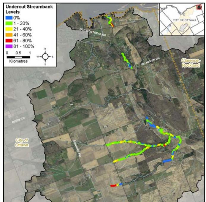
Figure 7 Undercut stream banks along Becketts Creek
