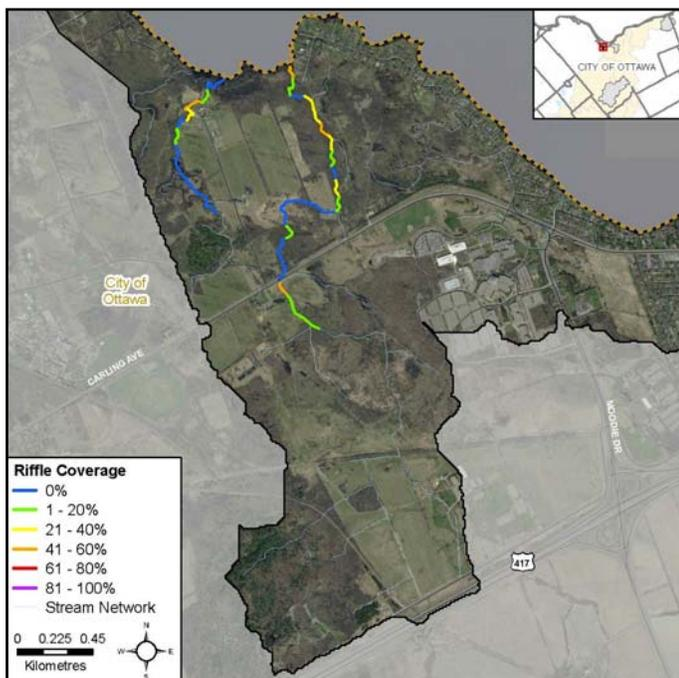
Figure 15 Riffle coverage along the Ottawa West Tributaries
