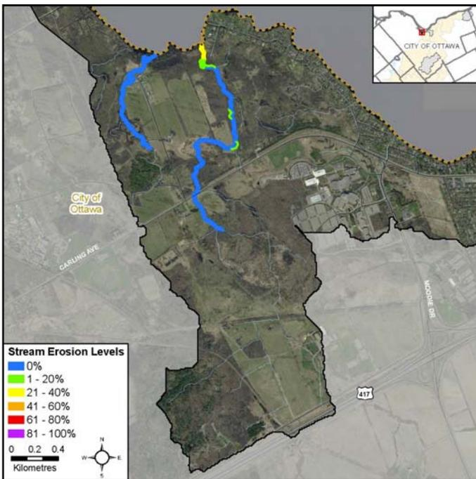
**Figure 6** Erosion Levels along the Ottawa West Tributaries
