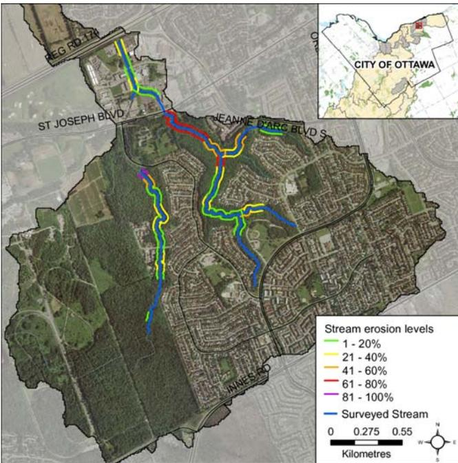
**Figure 4** Erosion along Voyageur Creek
