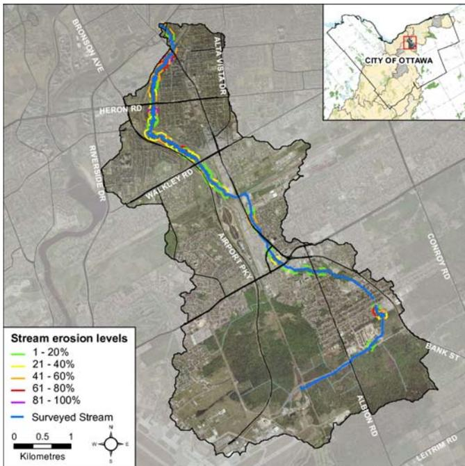
Figure 4 Erosion along Sawmill Creek
