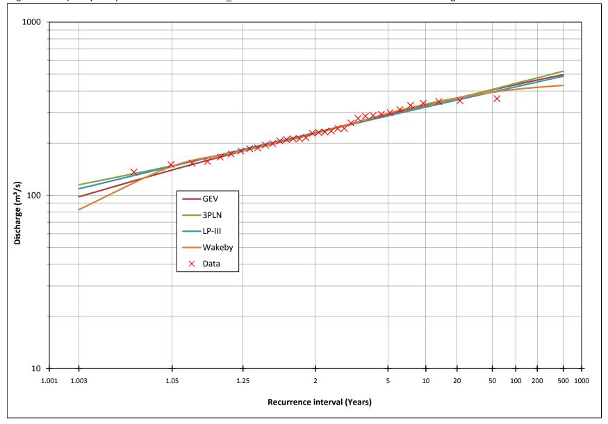
Figure B2 Frequency Analysis Distributions from CFA\_3.1 for the Rideau River Below Manotick Stream Gauge.
