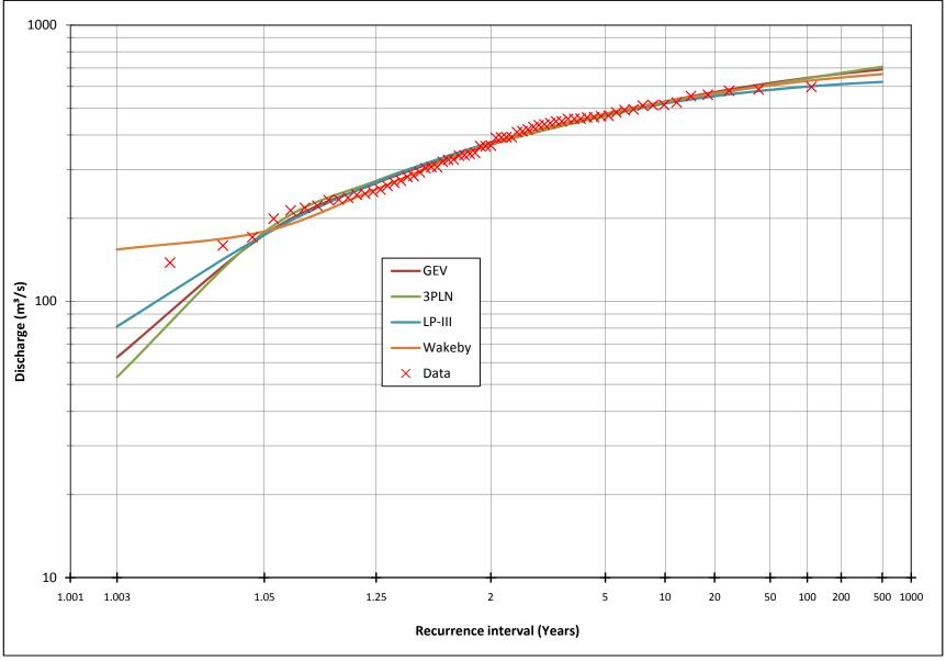
Figure B1 Frequency Analysis Distributions from CFA\_3.1 for the Rideau River at Ottawa Stream Gauge.
