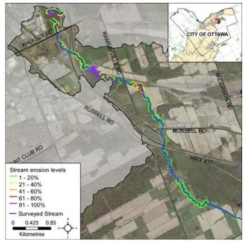
Figure 4 Erosion along Ramsay Creek
