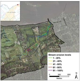
Figure 4. Erosion along Ottawa East Tributary
