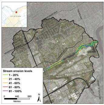
Figure 4. Erosion along Nepean Creek
