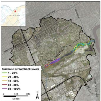
Figure 5. Undercut streambanks along Nepean Creek
