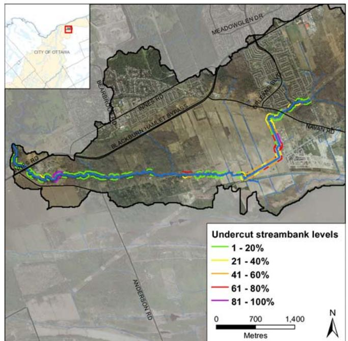
Figure 5. Undercut streambanks along Mud Creek
