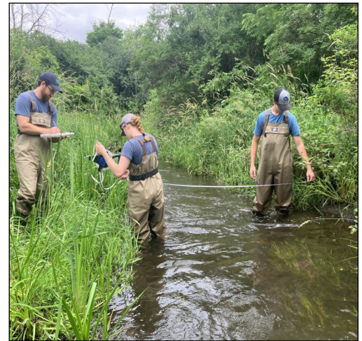
RVCA staff measuring wetted width during a stream survey.
