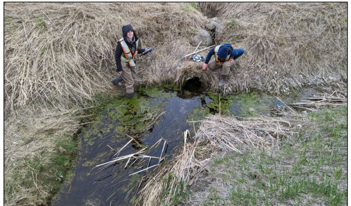
Volunteers using a multiparameter YSI probe to measure the water chemistry of a headwater drainage feature during a spring site visit
