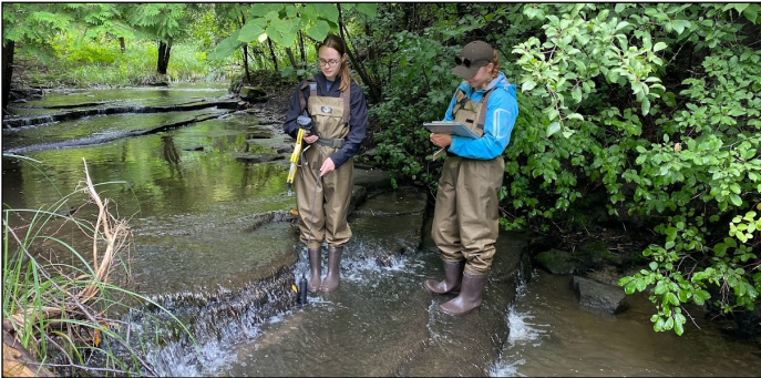
RVCA staff collecting water chemistry measurements with a multiparameter YSI probe
