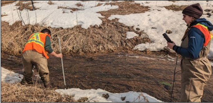
Staff collecting water chemistry measurements with a multiparameter YSI probe
