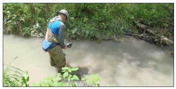
Volunteer collecting water chemistry measurements with a multiparameter YSI probe
