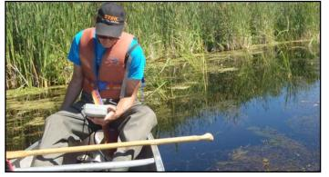
A volunteer collecting water chemistry measurements with a multiparameter YSI probe
