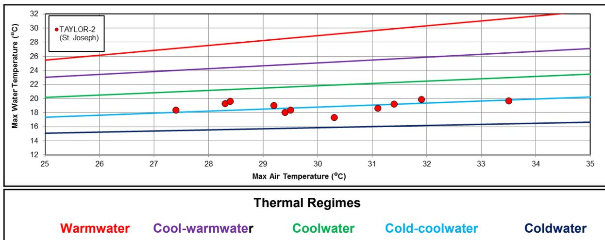
Figure 28 Thermal Classification for Taylor Creek with the five thermal regimes adapted from Stoneman and Jones (1996) by Chu et al. (2009): **Coolwater** category for the thermal site sampled on Taylor Creek
