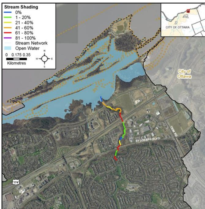
Figure 9 Stream shading along Taylor Creek
