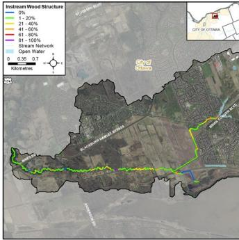
Figure 16 Instream wood structure along Mud Creek
