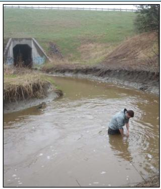
Temperature probe installation on Mud Creek upstream of Innes Road
