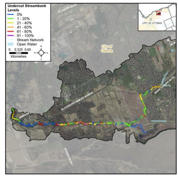
Figure 7 Undercut stream banks along Mud Creek
