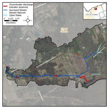
Figure 29 Groundwater indicators observed in Mud Creek
