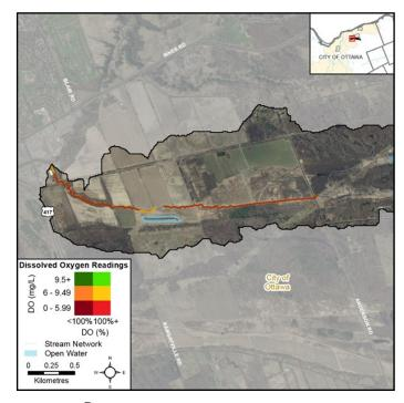
**Figure 25** Bivariate assessment of dissolved oxygen concentration (mg/L) and saturation (%) along Black Creek
