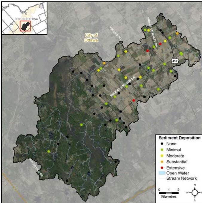
**Figure 38** Headwater feature sediment deposition in the Stevens Creek catchment
