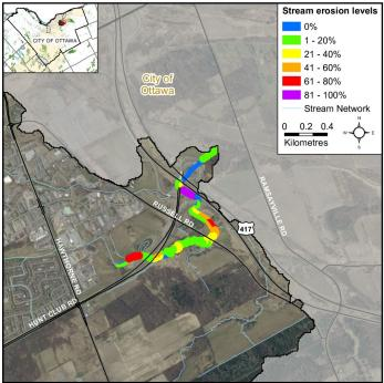
Figure 4 Erosion along McEwan Creek
