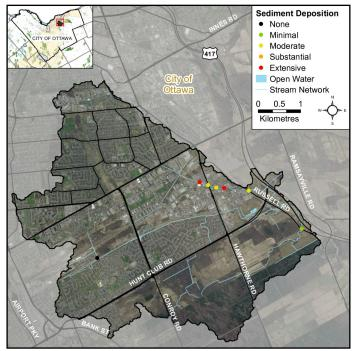
Figure 38 McEwan Creek HDF sediment deposition
