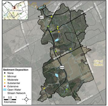
Figure 39 Graham Creek HDF sediment deposition
