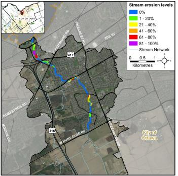
Figure 4 Erosion along Graham Creek
