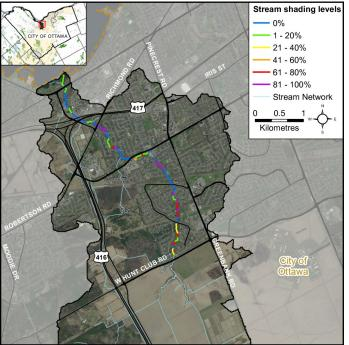
Figure 7 Stream shading along Graham Creek
