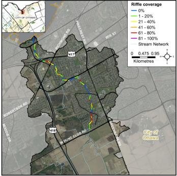
Figure 15 Riffle coverage in Graham Creek
