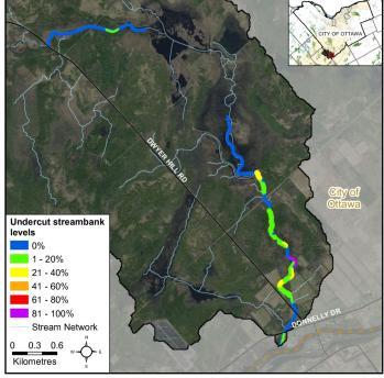
Figure 5 Undercut stream banks along Brassils Creek
