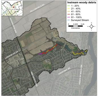
Figure 7 Instream woody debris along Barrhaven Creek
