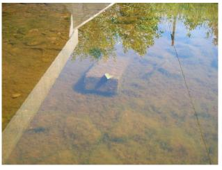
Photo of datalogger deployed in Stevens Creek on a block
