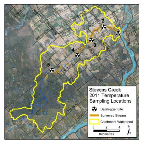
Five temperature dataloggers were deployed in Stevens Creek to give a representative sample of how temperature fluctuates and differs along the stream. The dataloggers were installed in April and retrieved in late September. Dataloggers are either secured to blocks on the bottom of a stream or attached to rebar secured to the bottom.
