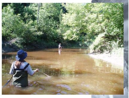
a photo is taken upstream. Water temperature is recorded to the nearest °C. Stream width is measured to the nearest tenth of a metre using the 60-meter tape, spread at right angles to the banks originating at water level. Stream depth is measured, using the metre stick, at the deepest point along the width of the
