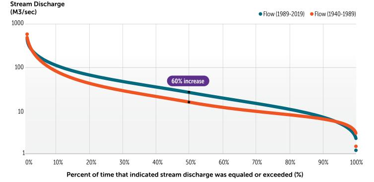
FIGURE 2.6 Flow Duration Curve for the Lower Rideau River (02LA004)
