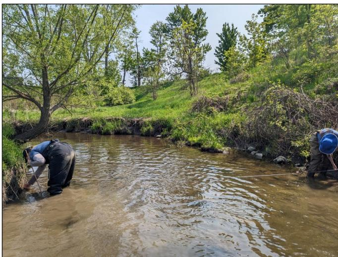
RVCA staff measuring stream width on Mosquito Creek downstream of Limebank Road
