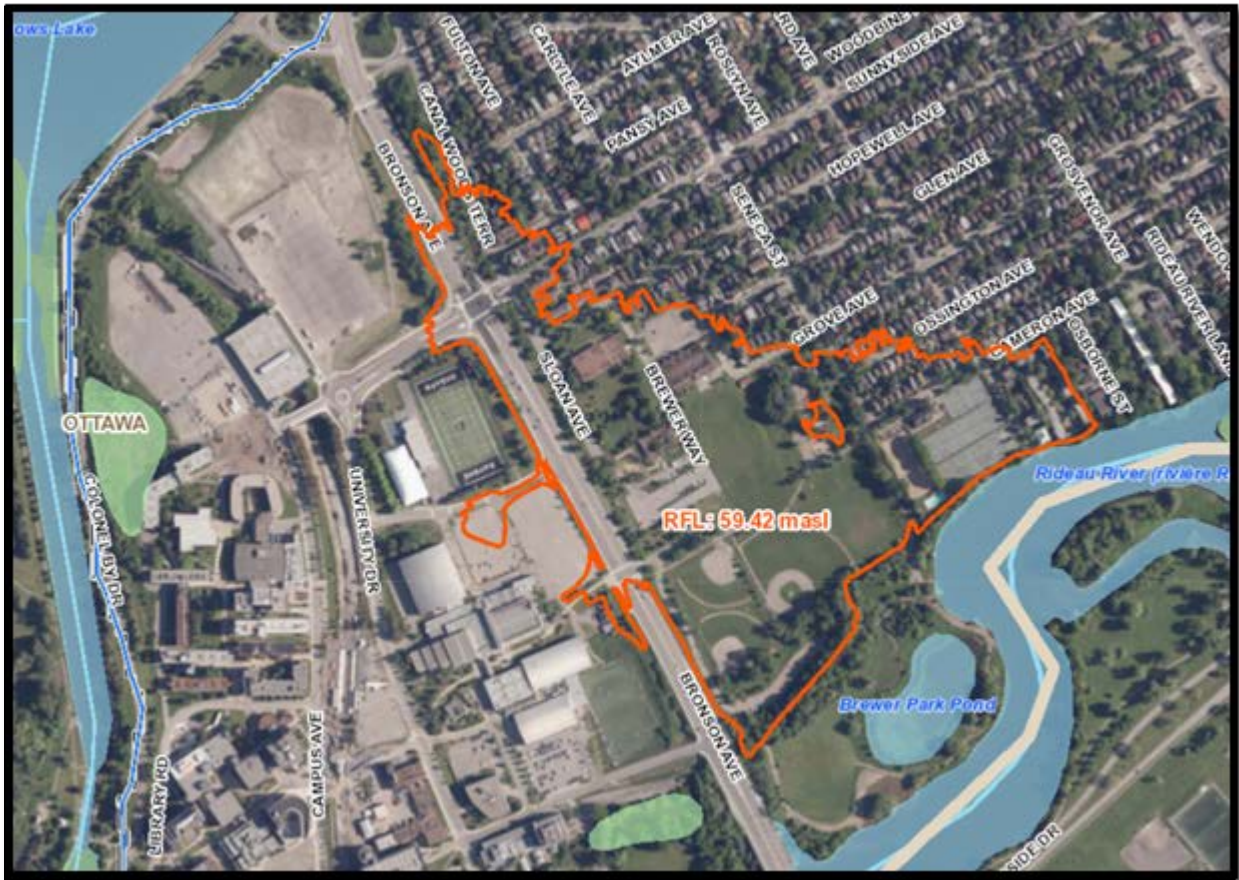
Schedule A: Mapping identifying approximate area of Brewer Park and Carleton University Flood Protection Area based on a regulated flood level of 59.42 metres above sea level
