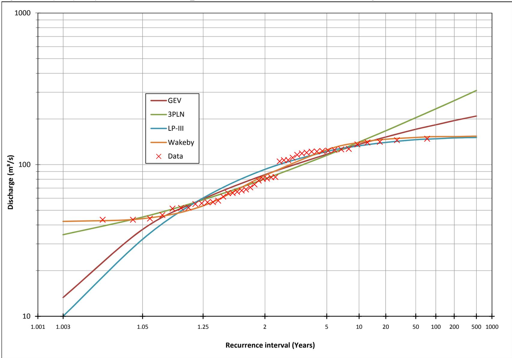
Figure B5 Frequency Analysis Distributions from CFA\_3.1 for the Kemptville Creek Near Kemptville Stream Gauge.
