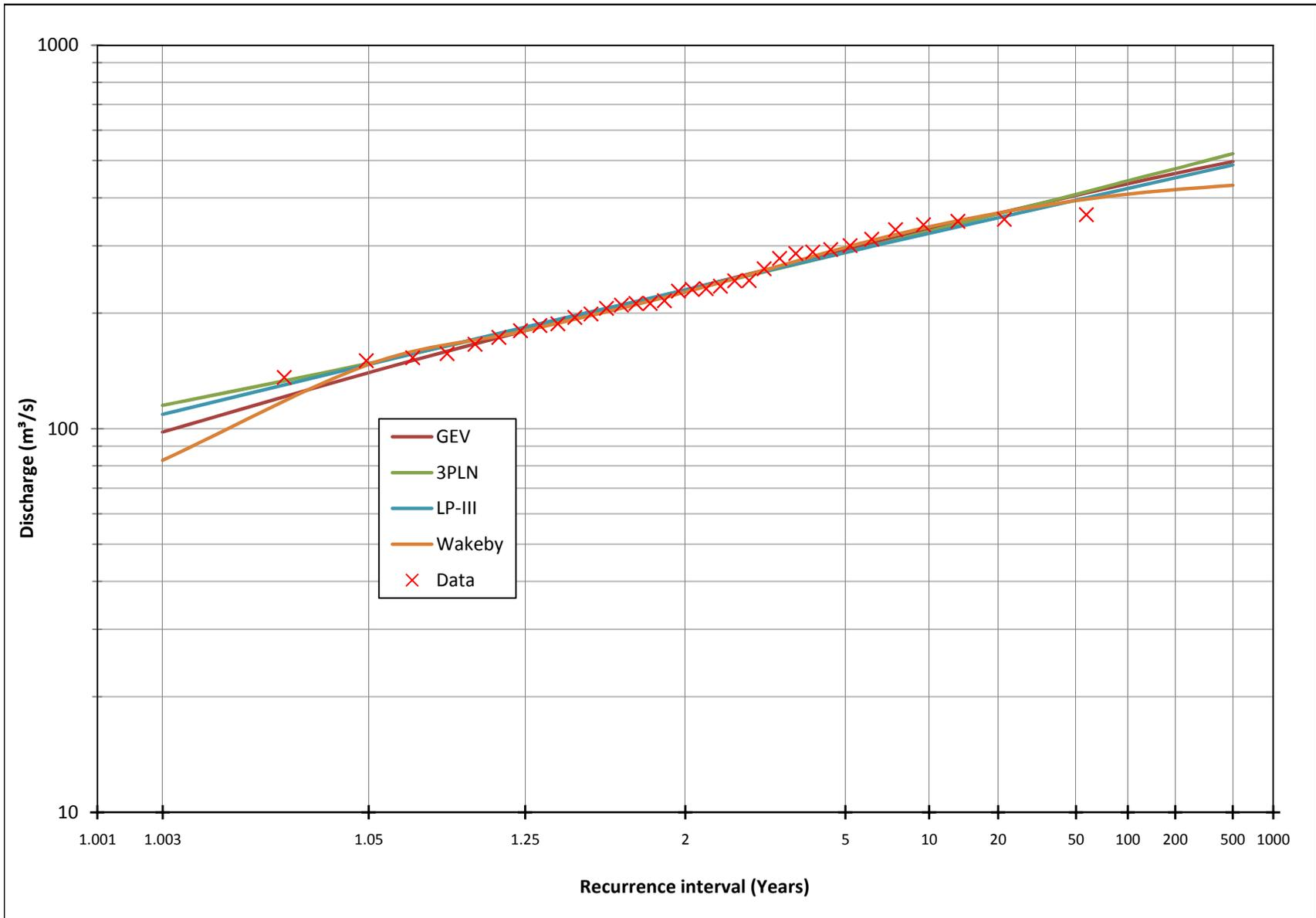
Figure B3 Frequency Analysis Distributions from CFA\_3.1 for the Rideau River Below Merrickville Stream Gauge.
