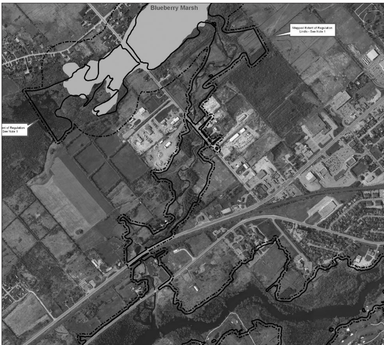
New Blueberry Creek Maps — the solid line is the updated floodplain and the dashed line is the updated regulation limits.
