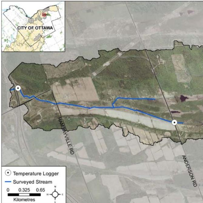
**Figure 18** Temperature loggers along Borthwick Creek
