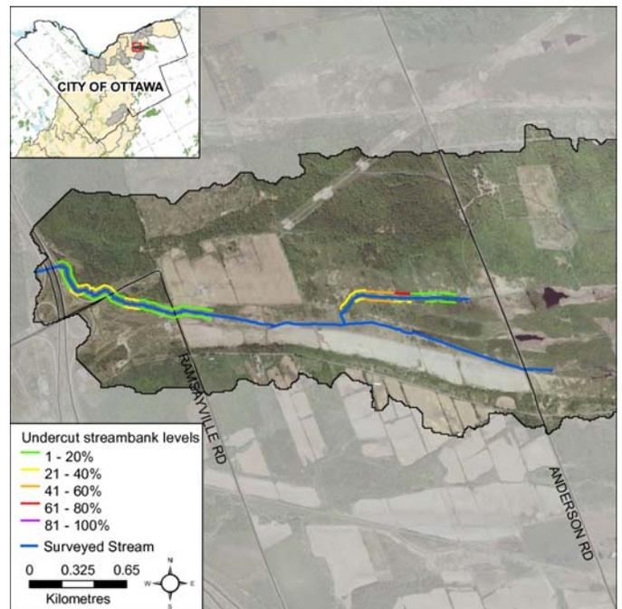
**Figure 5** Undercut stream banks along Borthwick Creek
