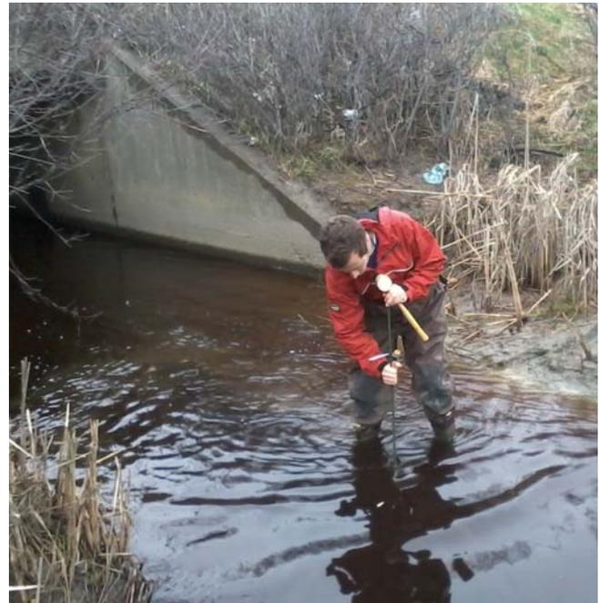
Temperature logger installed near Highway 417
