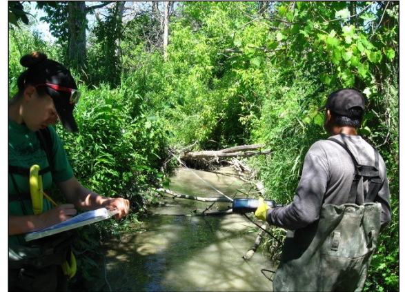
CSW volunteer measuring water chemistry using a YSI multi-parameter water quality meter while a
