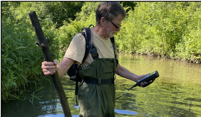
Volunteer collecting water chemistry measurements with a multiparameter probe.
