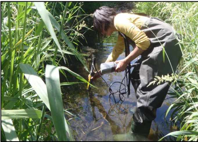
Collecting water chemistry measurements with a YSI probe on Nepean Creek
