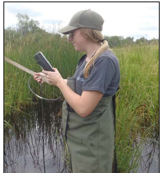
RVCA staff measuring water chemistry using a YSI multi-parameter water quality meter
