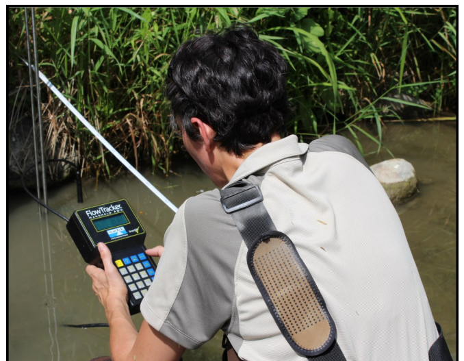
A SNC employee works to take baseflow measurements with highly accurate scientific equipment
